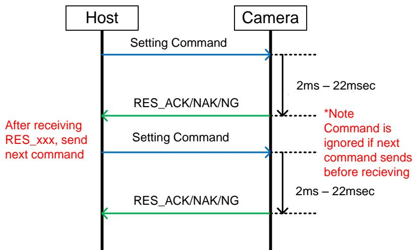
Command is usually a response within tens of milliseconds. However, **Factory Reset** and **Reboot** command is slow to respond because of the process of writing back parameters to non-volatile memory.
